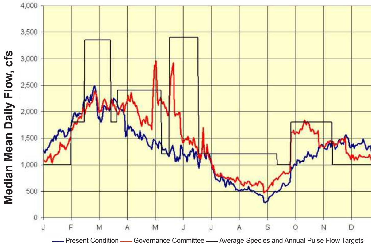
FIGURE III.3. Target Flows & Computer Generated Hydrographs for the Platte River
